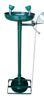
The pedestal mounted eye/face wash, with a plastic bowl, ABS plastic eye/face wash spray heads, an inline strainer, a stay-open 1/2" ball valve with a push handle and a hand foot control. The eye washer and valve assembly is pre-built and fully water/pressure tested to ensure no leaks and proper function which ultimately reduces installation time and gives the end contractor an added peace of mind. The Eye Washer unit that complies with EN 15154-1&2, AS 4775:2007 performance requirements.
